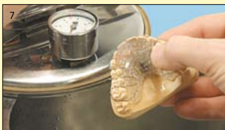
7 Polymerize in the pressure pot for 10 minutes at min. 45° C and a pressure of 2 bar.
