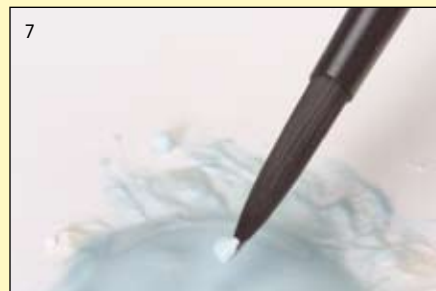
7 The optimized springiness restores the shape of the brush tip immediately after picking up ceramic material. Additionally, the respective quantity can be easily assessed thanks to the contrast.
