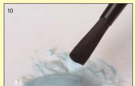
10 The spatula shape does not reduce the stability of the brush hair; hence less time is required for applying the ceramic material to the framework.
