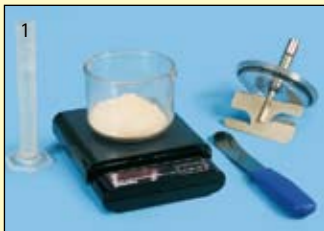
1 Weigh resp. measure plaster and water to obtain constant results.
