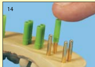
14 The thicker end of the Master-Pin sleeves is put on the Master-Pins.
