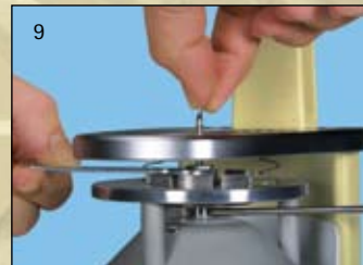
Drills are exchanged without the need to open the unit.
