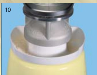
Any resulting plaster particles are automatically collected by the projecting collecting tray.
