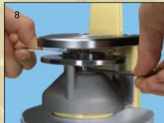
Drills are exchanged without the need to open the unit.
