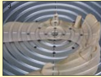
Guidelines on the model table allow specific alignment of the model for exact planning of pin holes.
