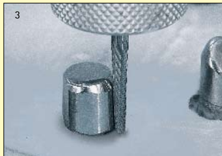
3 The crowns are milled quickly using Brealloys C + B 270 and the 2° NE profile bur.
