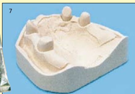
7 The exact expansion control offered by Brevest M1 is the prerequisite to produce precision-fit CoCr restorations.
