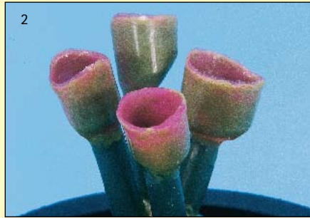
2 A max. wall thickness of 0,3 - 0,4 mm must be ensured.
