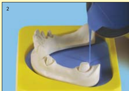
2 Fluid-Rock base stone is directly poured into the model former without using a vibrator. Perfect flow characteristics allow to obtain models without any bubbles.
