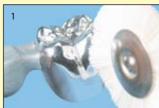
1 The low hardness facilitates milling, shaping and polishing.
