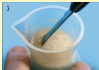
3 Mix liquid and powder to obtain a creamy consistency which will make processing easier.
