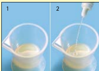
1 Mix Performance LiquidColdCuringPolymer in the ratio of 4 drops of liquid to 0.1g of powder.
