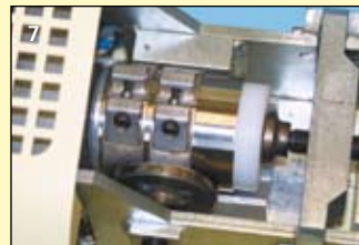
The muffle is placed in the thermopress 400 and fixed by means of the screws. Then the injection molding operation is initiated.
