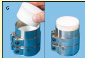
Tighten the screw of the metal sleeve and finally insert the plastic block to counteract pressure.
