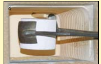
In order to melt out the wax heat the muffle in an oven at 900°C and then allow to cool.
