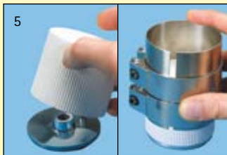
Replace the muffle on the metal base and surround with the metal sleeve. The metal sleeve should grip only the muffle.
