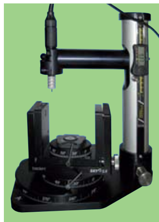
SKY5X coordinate table for the fabrication of a drilling template and the placement of drilling sleeves. REF SplanX02
