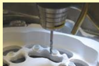
The right angled, flat headed burs provide a good seating surface on implant platforms.
